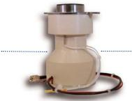
New 25 mm UltraFast BiPolar TOF detector
